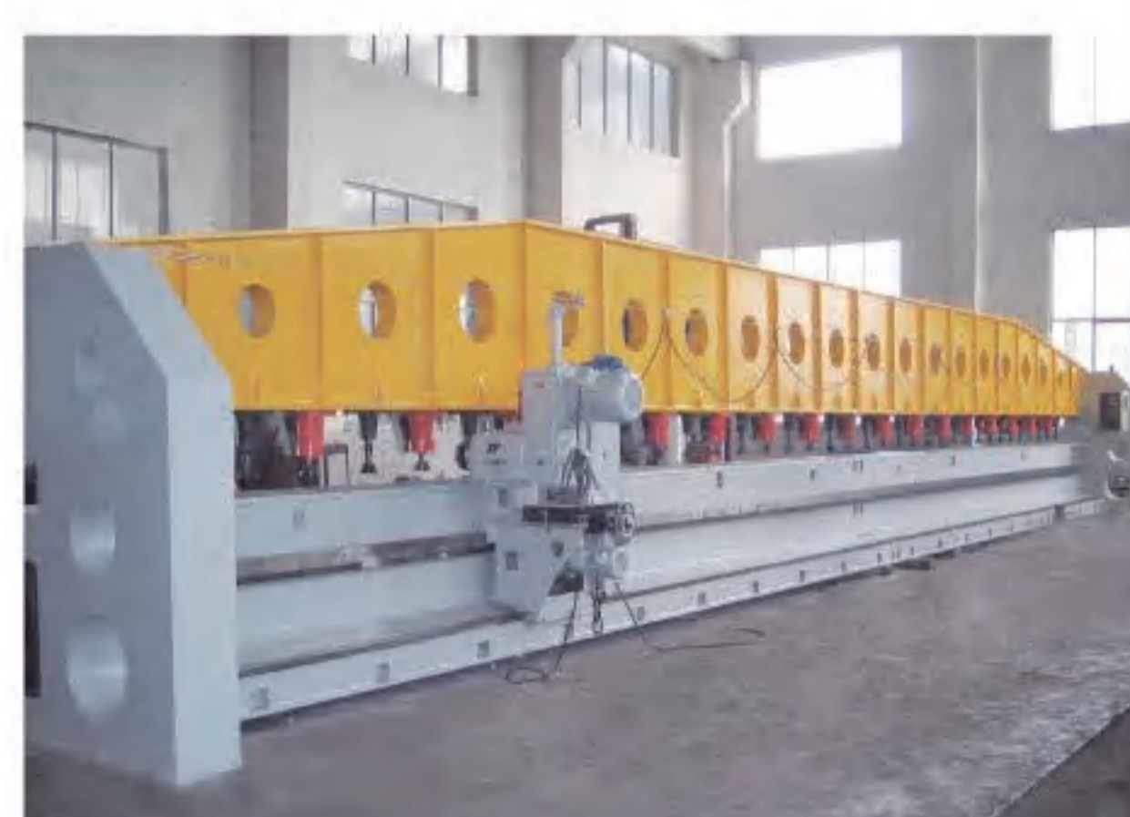
15米出口铣边机 Exported edge milling machine with 15 meters
