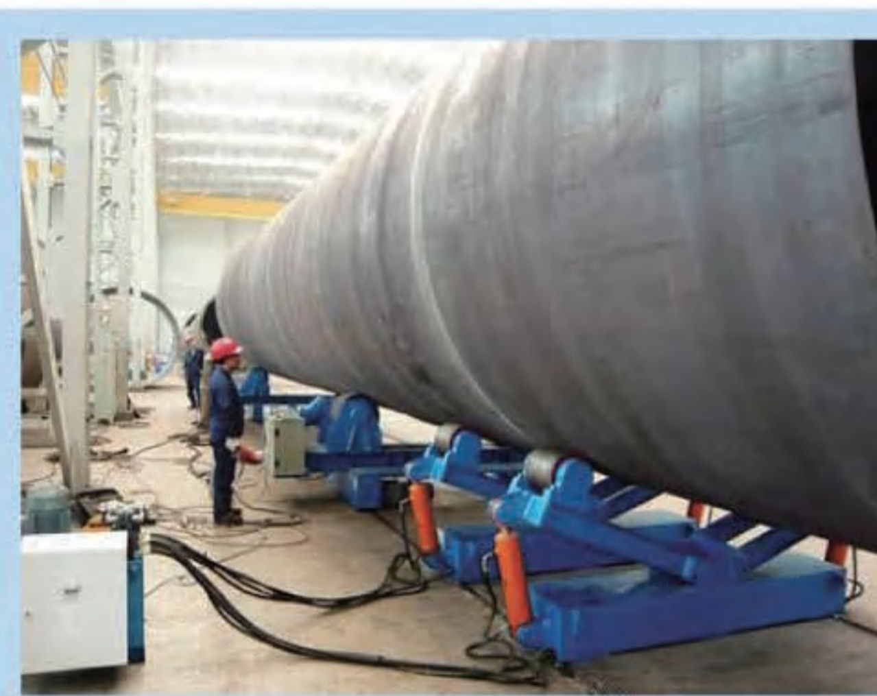
塔筒内外环焊接流水线 Welding line of outer circumferential seam
