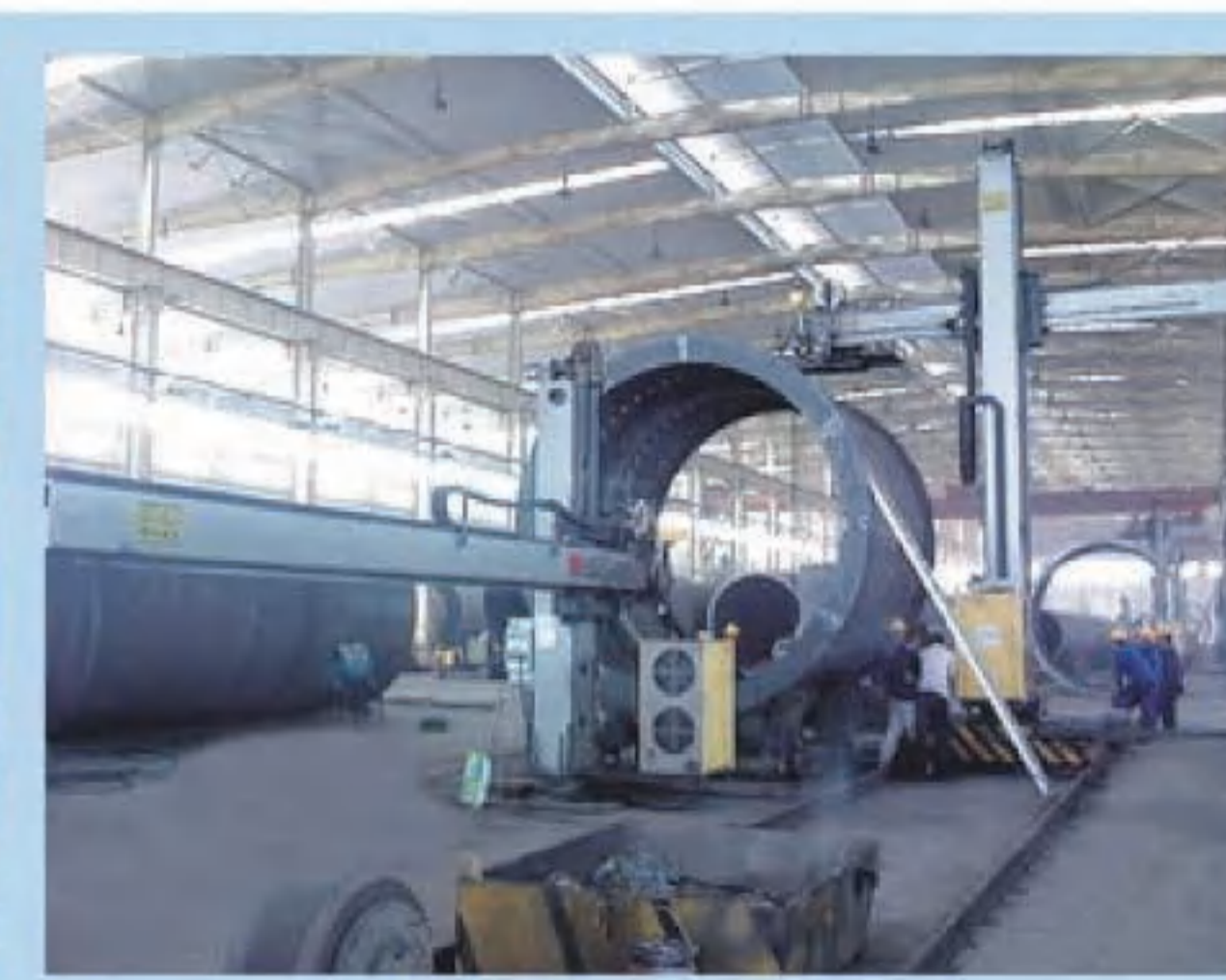
塔筒内环焊接 Inner circumferential seam welding
