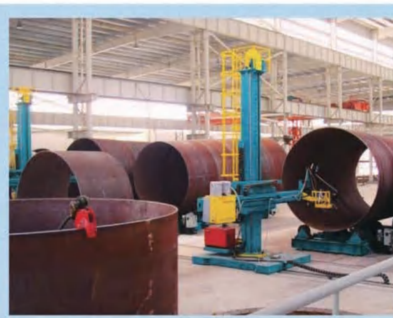
塔筒内环焊接 Inner circumferential seam welding
